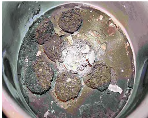
The bomb reduction and casting processes create lots of scrap that has to be dissolved and recycled back to pure metal
